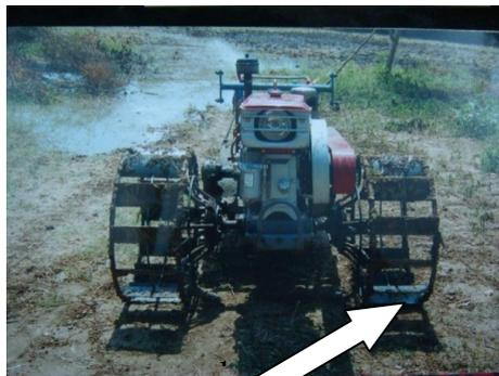
Figure 11: The arrow pointing to the steel link connecting the central rotor and the tilling wheel with heavy duty blades
